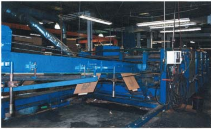
Rebuilding the EMBA 240 flexo folder-gluer has increased running speed by 50 percent.
